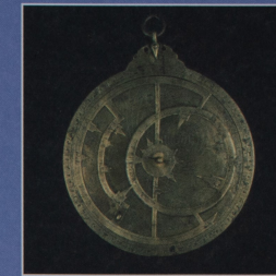
Brass astrolabe, Iraq. Dated 927/28, this astrolabe was used for observing planetary movements and for navigation. It is the oldest astrolabe in existence.
