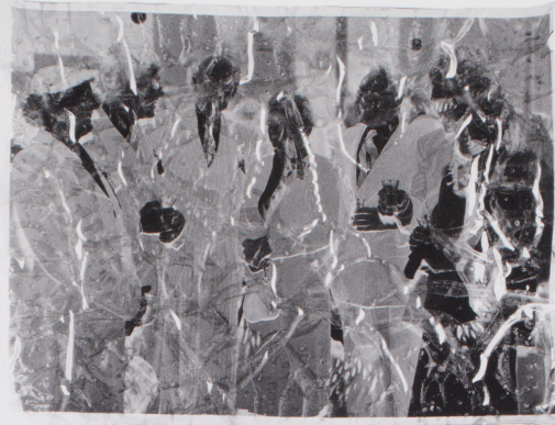
An example of degraded acetate negative film showing buckling, blistering and channelling of the image surface.
