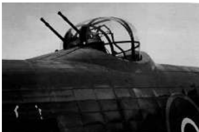
Lancaster 111 Mid Upper Gun Turret. From: http://www.ian.com.au/contact/images/lancaster/turret_u.jpg
